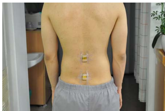
Fig. 3. Photograph of 2 microelectromechanical system inertial measurement unit transmitters attachment locations L1 spinous process and between posterior superior iliac spine.
